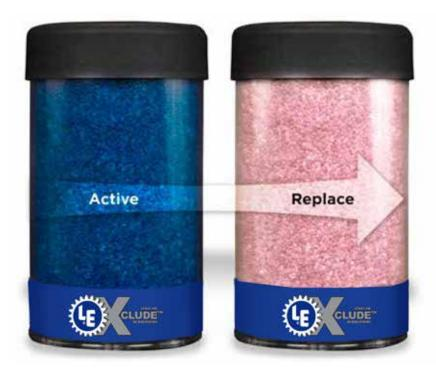
If the system was not previously equipped with a desiccant breather, it is normal for the first unit to change color relatively quickly on the initial installation. This means the product is working to remove existing contaminants already in the gearbox or reservoir, and its life will be shorter than typical. Subsequent units will increasingly provide longer life.
